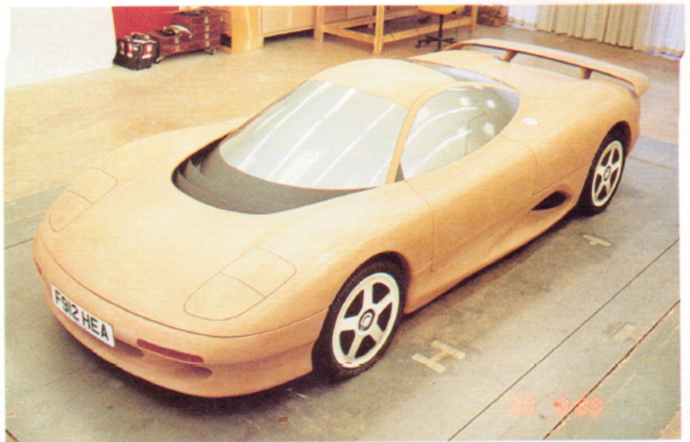
The finished full-size clay, painted Dynoc representing window areas. Photo: P. Stevens.
